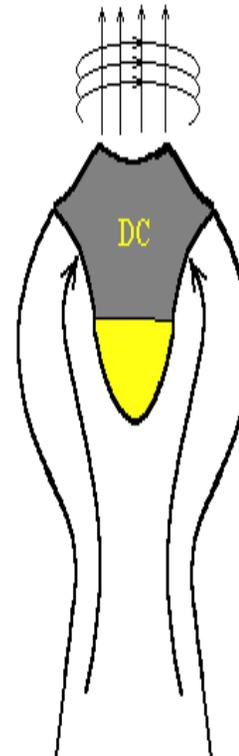
Another example concerns the use of a *static* tornado chamber inside the chimney to create a structure of exhaust gases in a form of a twirling tornado-like column. Such a column will be a very stable dynamic formation, tough to be destroyed by wind, and will lift exhaust gases much higher, which is necessary for a good dissolution of them in ambient atmosphere (to decrease their possible harmfulness at high concentrations).
