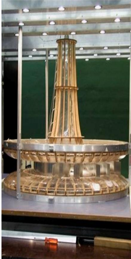
*Tornado chamber built in Wind tunnel of the Hamburg University, Germany.*
