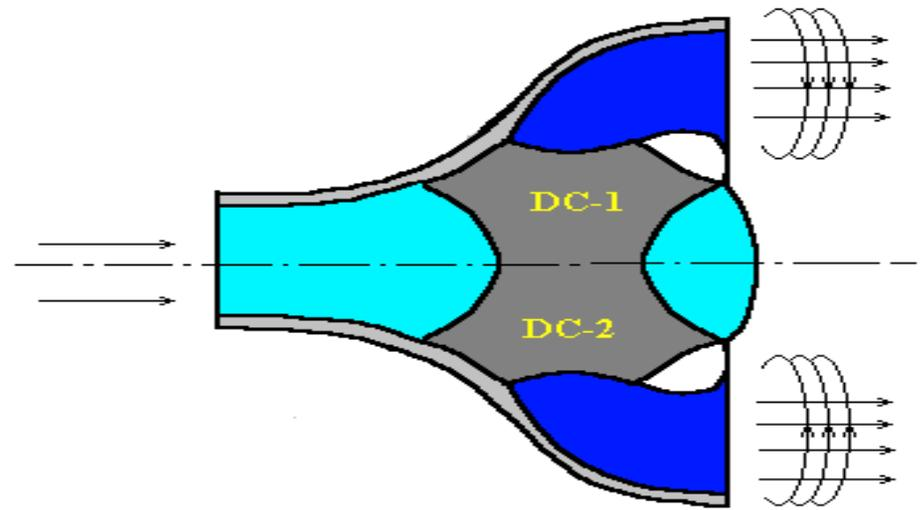
Tandem of two diagonal TC with intake helices is shown. In this embodiment all axial forces are compensated. The torsion moments of two flowing out whirling streams are also compensated.
