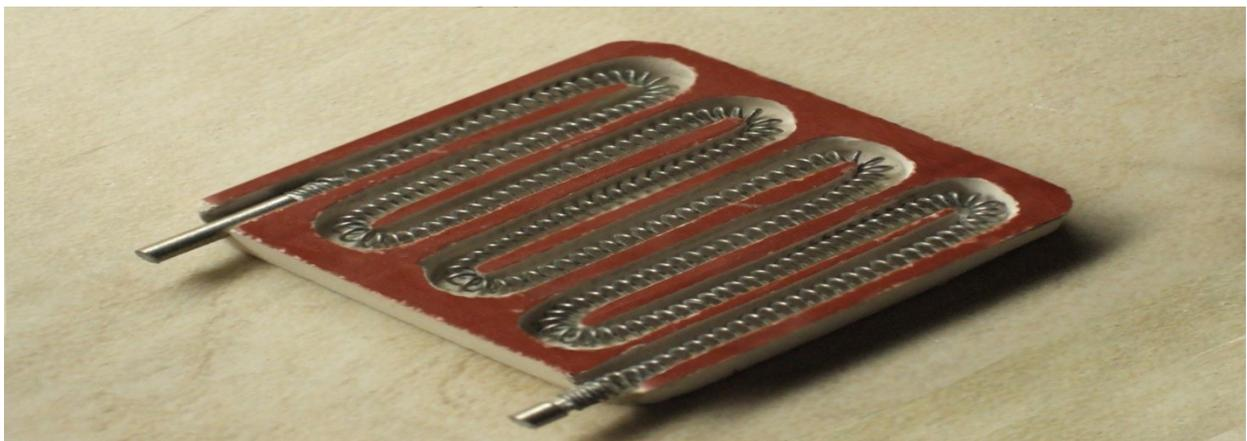
Fig. 2. Heating element before pressing (with fulfilling with a quartz sand) and sealing it into a sleet into the copper cube)
