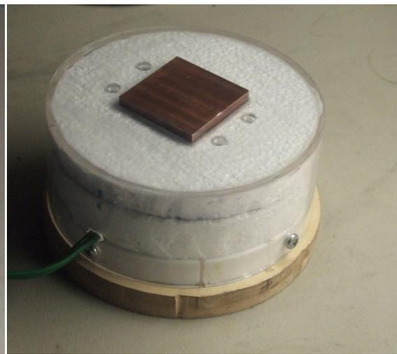
Fig. 3b. PC processor imitator with attachment holes.
