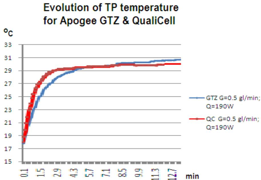
Fig. 5. Development of temperature of TP after instant turning on of heater for a given electric power.
