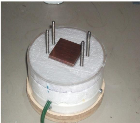
Fig. 3a. PC processor imitator with attachment bolts.
